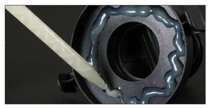
A leading UK designer, manufacturer and integrator of precision control components and systems uses Robnor PX800F, a fast curing multi-purpose epoxy adhesive in production.
